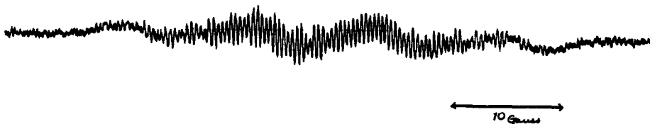
FIG.2 ESR spectrum of PAC in dilute chloroform solution at room temperature.
